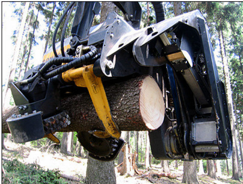
The RFID-enabled harvester staples tags into logs automatically to help track timber moving through the processing line.
